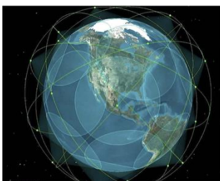
Globalstar's current constellation design. (Source: Globalstar Dec. 30, 2025, FCC filing)
